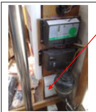
The final Green addition was an Ultrasonic antifouling system now fitted to avoid the use of toxic antifouling solutions. By transmitting a variety of ultrasonic frequencies through the hull, this inhibits the attachment of barnacles and other marine life that foul a ship's hull. The system consists of a transducer which is bonded to the hull, and a control box to produce the range of frequencies required.
